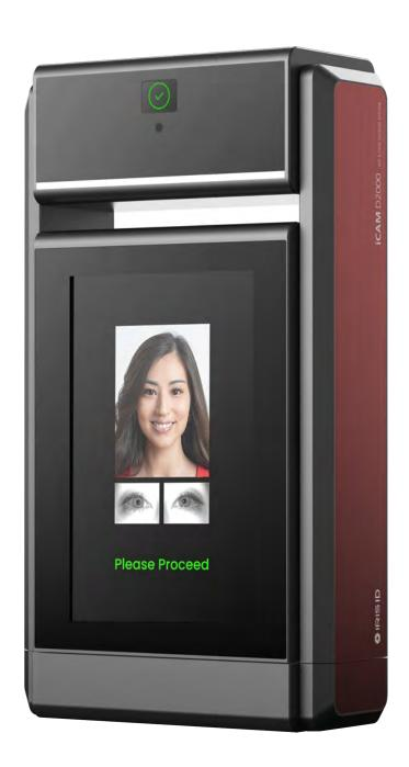
Compact, insightful, and unparalleled quality in biometric performance, Iris ID's iCAM D2000 represents a new class of fused iris and face identification systems. Flexible capture distance ranging from 50cm to 1.0m, iCAM D2000 provides an ergonomically intuitive user experience while delivering high quality iris and face images for enrollment and identification. With focus on usability and dimensions the iCAM D2000 is ideal for identity, travel and access solutions.
